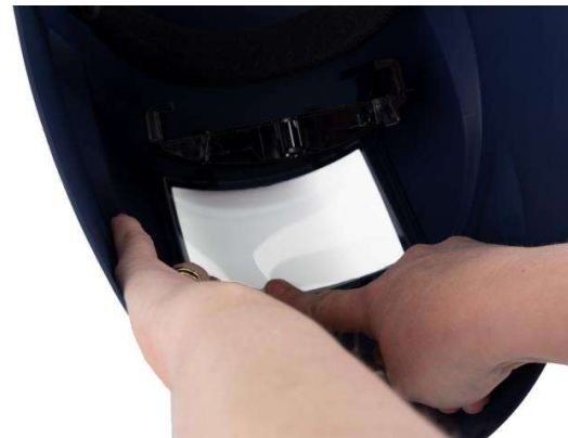
6.4 Fit the protective lens. Fit the holder. Tighten the screw.
