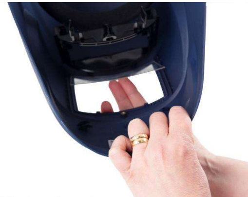
6.3 Release and remove the outer protective lens
